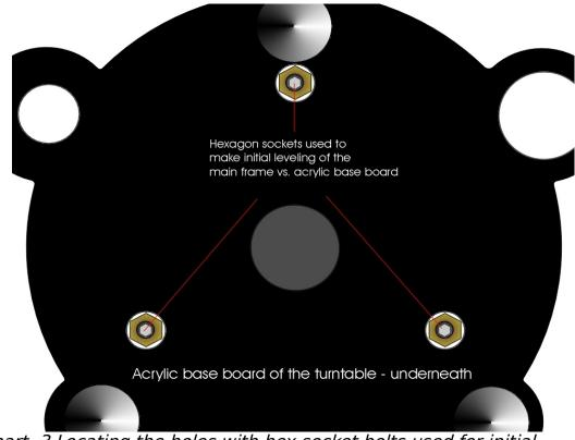
*Chart 3 Locating the holes with hex socket bolts used for initial leveling.*
