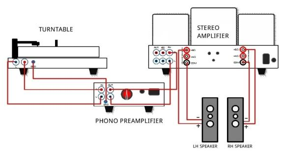
*Chart 4: Scheme of the wiring of the turntable within Audio – Stereo system, incl. phono preamplifier.*
